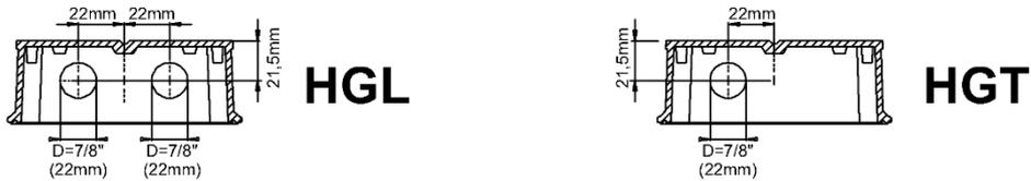
**Fig. 19: Dimensions – Plastic enclosures for conduit hubs**
