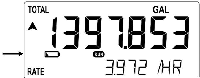
**Fig. 8: Example of low-battery alarm**
